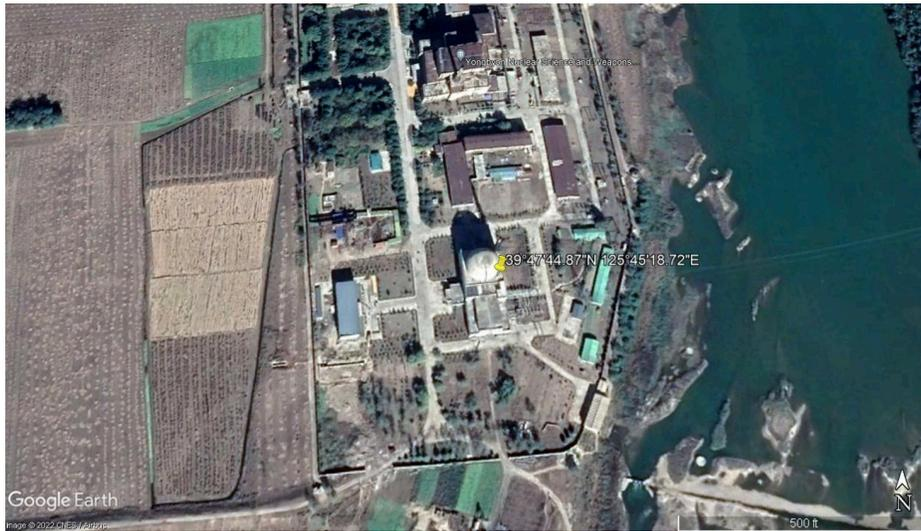
The Taecheon 200MW Graphite-Moderated Reactor (태천 200MW 흑연감속로) is located in Taecheon County, North Pyongan Province at 39°55'40.13"N, 125°34'13.49"E. Its construction began in 1989, but it was abandoned in the 1990s. It is unknown whether any personnel are deployed at this facility.<sup>124</sup>
